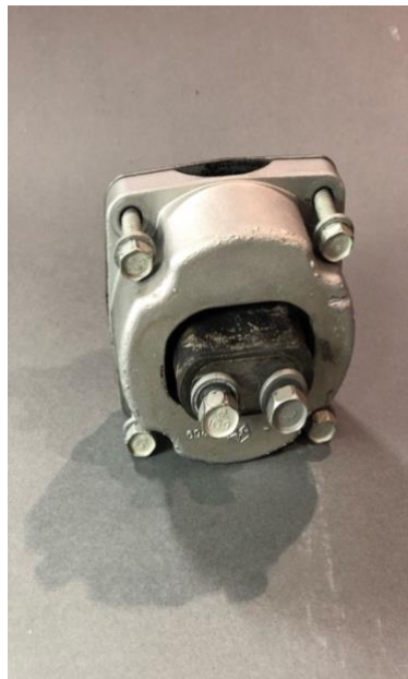
Install Picture 5- Factory transmission mount removed
