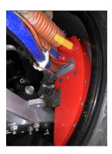
**Step 8**: Now that you know where your brake duct hoses will be routed, it's time to install your hose route bracket. While keeping the hoses running level from the brake duct adaptor plate, hold the bracket up to the frame of the vehicle. Move the brake duct hoses and mark the holes in the bracket at the desired location. Use a 5/32 drill bit and drill the marked holes. Use included 5/32 rivets to secure the bracket to frame. See Figs. below.
