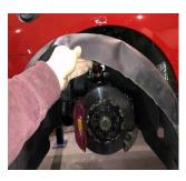
**STEP 2:** Use a 5/32 drill bit and drill out the rivets holding the factory brake duct. You can also use dike cutters to cut the rivets once they are loose. Remove the factory brake duct. See Figs. below.
