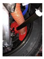
**STEP 7**: Now that the rear brake cooling kit has been installed, put the wheel back on and inspect that the hoses are not in contact with the wheel. Adjust if necessary. See Figs. below.
