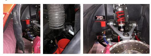
**STEP 5:** Use a 19mm wrench to remove the aft wheel bearing bolts closest to the caliper. Slide the shroud into place and use a 19mm socket on extension to secure the (2) included ½"-20 bolts. Torque bolts to 90 ft.lbs. (The brake line banjo fittings on the caliper will need to be at the 12:00 position if not already).
