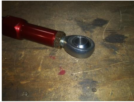
Fig. 9 (ALWAYS TIGHTEN JAM NUTS)
