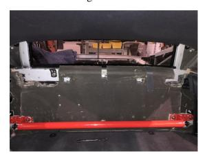
**STEP 8**: Now that the racing harness mounts are in place, re-install all of the interior panels except for the carpet panel that goes against the firewall, you will need to use masking tape and mark where the carpet panel will be notched out to fit the racing harness mounts through on both sides. Use a Dremel and take small cuts from the carpet panel so you have a precise tight fit in the end. See figs. below.
