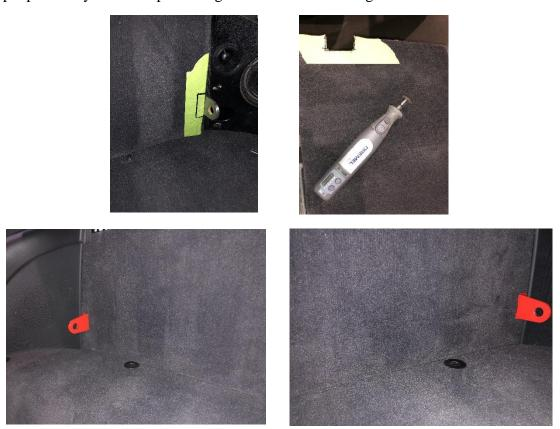
**STEP 9**: Install the racing harness bar and apply blue loctite to the M14 bolts before tightening. Finally, install racing harness onto the bar and the racing seat.
