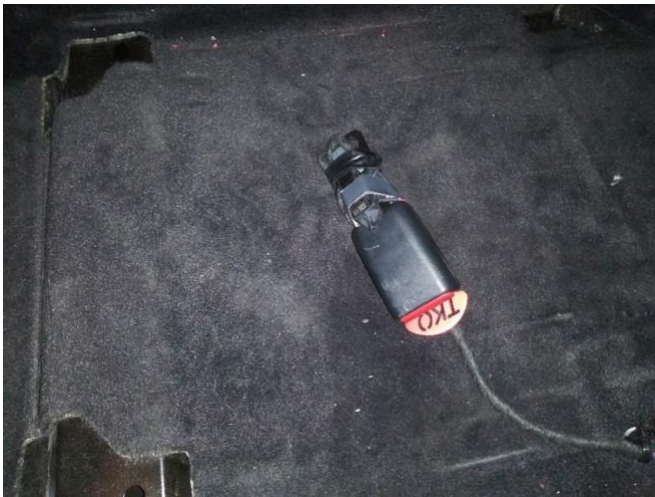
Fig. 20 Seat belt simulator installed into the seat belt latch
