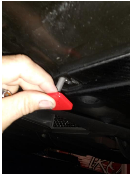
Fig. 15 - Viper ACR models with diffusers, you will have to notch out the front edge of the carbon fiber diffuser strake mount to install the M8 stud plate on the inboard side. Check the fit before the final installation.
