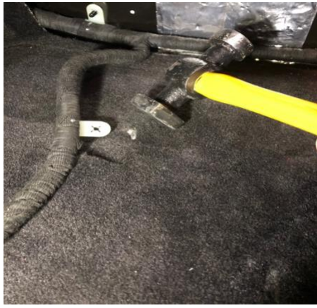
Fig. 8 - knock over wire route pin
