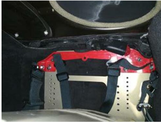
Fig. 19 - Lap belts and sub straps installed, racing belt mounting bracket installed onto the seat mount and ready for the seat to be installed to adjust the belts prior to the final installation. Some factory Viper seats come with sub strap routes in the base of the seat. If your factory seat has no sub strap routes, you can route the sub straps around the front of the seat.
