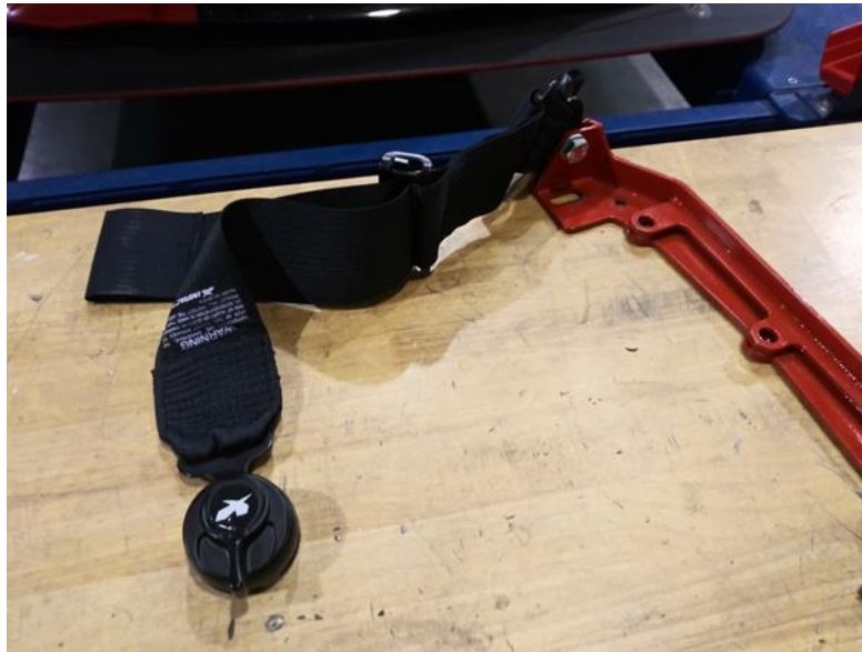
Fig. 16A - Make sure you install the cam lock side on the inboard side of the belt mounting bracket. The cam lock on the inboard side is recommended to reduce the risk of damage to the threshold plate and rocker damage when disconnecting the belts.
