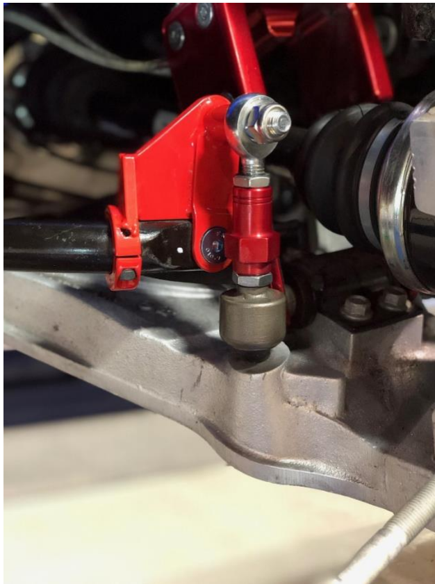
REAR SWAY BAR LINK WITH EXTENSION BRACKET INSTALLED ON REAR SWAY BAR
