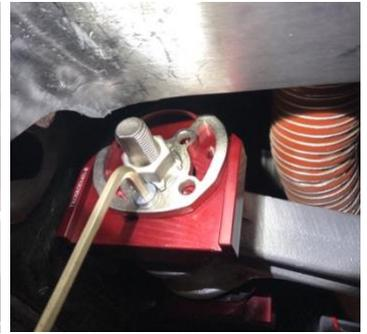
**INSTALLING THE LOCKOUT PLATES IN POSITIONS 2&6:** In these positions, the lock out plates were designed differently to accommodate for the lack of working space. They function the same as the others and will be installed the same. However, the control arm bolt gets bolted to the eccentric plate using a 4mm allen key. Once these black bolts are screwed in, they will not need to be removed to make adjustments. You will make adjustments the same way as the others. See pictures below.
