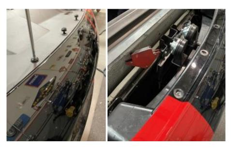
STEP 2. Push down on the plastic grill and insert the tow hook. Rotate the tow hook 90 degrees to allow for the round tube crossmember to sit in the lower clamp. Place the upper clamp over the round tube crossmember (on some Vipers you may need to give the AC condenser a slight push to allow for the upper clamp to clear) and align the keylock groove on the upper and lower clamps and push into place.
