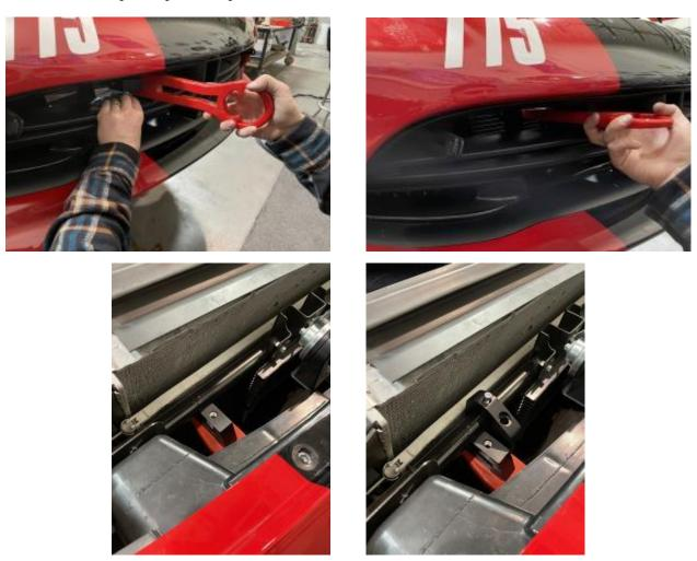
STEP 3. Using a 10mm Allen socket, snug the clamp so that the tow hook is still adjustable. Step back and ensure that the tow hook is parallel to the ground. Once you are satisfied with the position of the tow hook, tighten the clamp. Use a 5mm Allen socket to tighten the set screw enough to mark the round tube crossmember. Remove the clamp and use a .228 drill bit and drill a hole for the set screw to pass through where the mark on the tube is.
