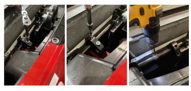
**STEP 4.** Align the clamp with the drilled hole in the round cross tube crossmember and tighten the clamp. Tighten the set screw until it passes through the round tube crossmember and the socket cap sits flush in the clamp. Reinstall the radiator cover and car to its original condition.
