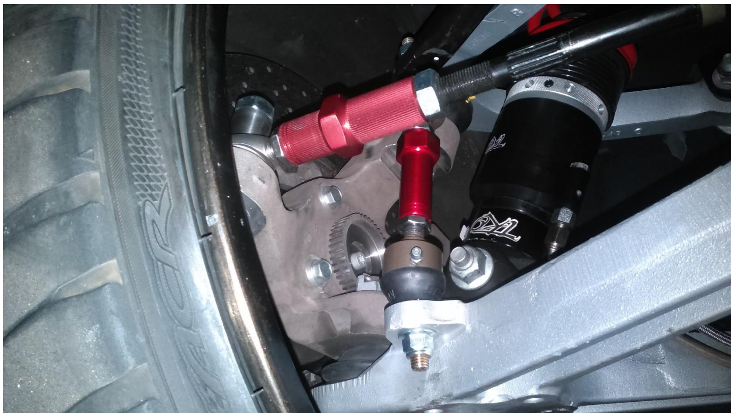
FRONT SWAY BAR LINK INSTALLED ( TKOSROD1390K 2003-2017 LOWERED DODGE VIPER SHOWN IN PIC )
